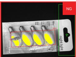
A package of light bulbs is inspected to confirm that all 4 bulbs are present and that none of the bulbs are broken.
