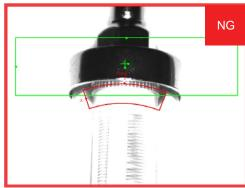
A fuel filter assembly is checked for the presence of an O-ring installed in the proper location before final packaging.
