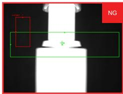
A lotion bottle is checked to confirm that the pump dispenser is in the locked position before the bottle is packed into a carton.
