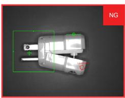
The distance between the two halves of an enclosure is measured to verify that the electrical plug has been assembled correctly. An open plug will cause a failure in the downstream packaging equipment.
