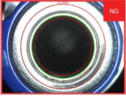
A wheel hub bearing is checked for the presence of quality control (QC) marks before moving to the next stage of assembly. The absence of the QC marks indicates that the hub bearing has not yet been inspected.
