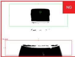
In-Sight vision sensors allow you to perform multiple inspections with each image. In this example, a bottle passes in front of the sensor, and both fill level and cap assembly are validated before the product is packaged.
