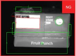
Inspections on a juice box verify that the date/lot code has been printed, confirm the safety seal is intact, check for the presence of a straw, and confirm that the flaps are fully secured.
