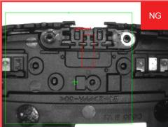
The presence of a rubber gasket attached to a molded plastic part is verified before an automated final assembly step.
