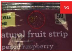
A color pixel count tool verifies that the correct fruit snack flavor is present to ensure that it is packaged in the correct order.
