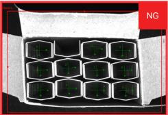
A pattern counting tool is used in this example to inspect the carton and to verify that the correct number of staple strips have been added.
